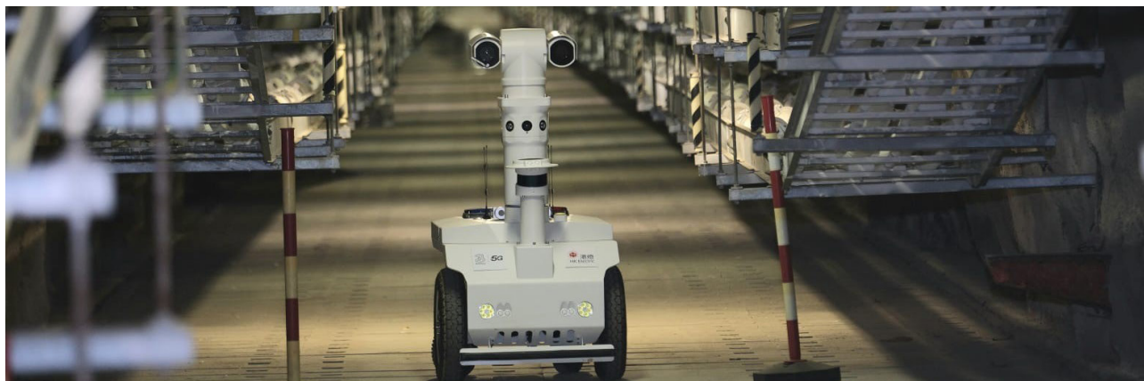
AI robot can detect the environment in confined spaces with built-in cameras, as well as gas, humidity and temperature sensors. 人工智能機械人可透過內置鏡頭，以及氣體、濕度及溫度感應器，探測密閉空間內的環境。
